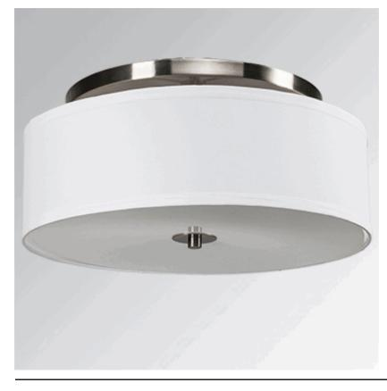
7.5"x16" Brushed Nickel Pendant, direct wire, three GU24, with 16"x16"x5" White Linen Hardback shade with bottom white acylic diffuser. Recommend three 1100 lumen LED bulbs with GU24 base.
